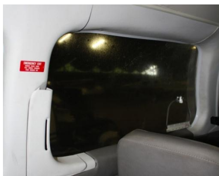
Figure 16: view of the emergency exit (Not used after the crash).
