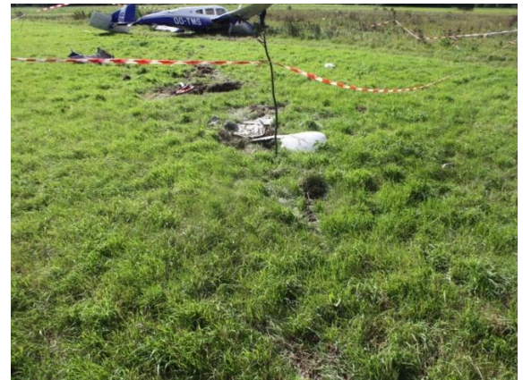
Figure 10: last impact traces with airplane in background
