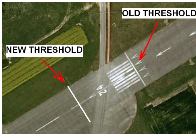
Figure 6: View of the new and the old threshold
