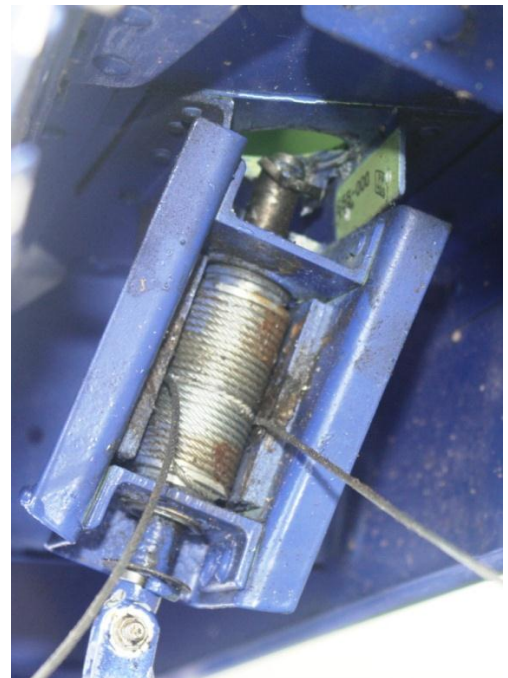
Figure 13: Picture of the rudder trim position.
