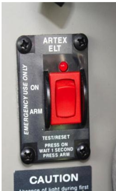
Figure 17: ELT Switch installed on Dashboard.
